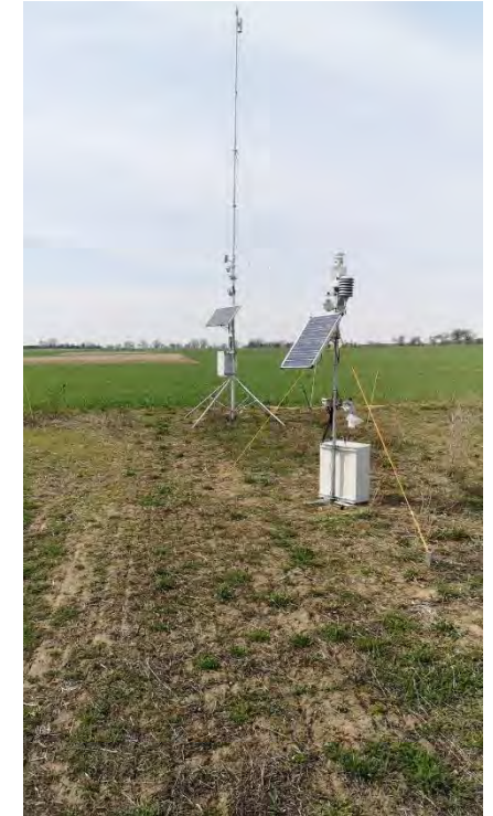
Transmission tower & LoRa Gateway
